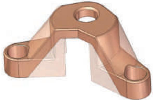
Figure 3. Making a significant change by rotating features initially extruded is easy using synchronous technology. Live Rules recognizes symmetry so an edit can be made to either vertical support.
