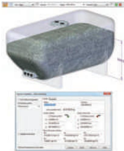
The example in figure 16 shows a portable tank containing a set volume of fluid. Goal Seek will automatically optimize the height of this fluid off the floor based on that defined volume.
