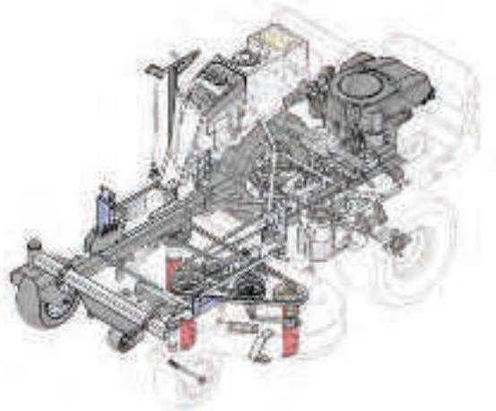
Figure 9. Solid Edge can produce a complete digital design complete with sheet metal, machined and supplier components as well as frames, wiring, and tubing designs. (Model image courtesy of the Magic Circle Corporation)
